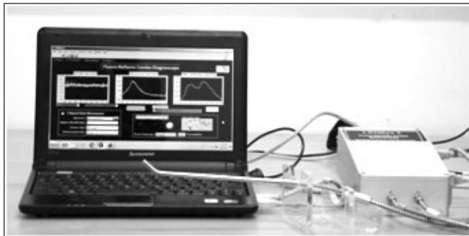
Figure 1. A USB powered, LED based combined fluorescence and diffuse reflectance system capable of providing automated diagnosis.
